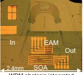
WDM photonic integrated circuit developed in this lab.
