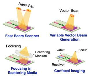
Fig. 1 Applications of adaptive lightwave synthesizer circuits.
